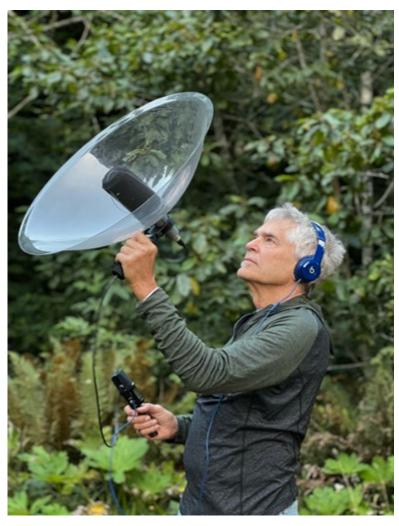
Above: The parabolic dish focuses the sound waves onto the tip of the microphone, and the recorder/amp processes and stores the signal with a time stamp. Photo courtesy of Robert Childs.
