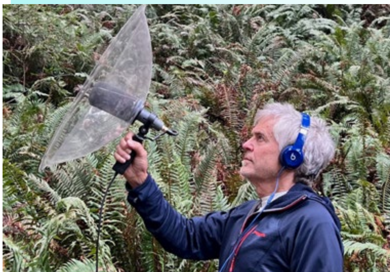
Left: Robert holding a parabolic dish to record bird sounds. Photo by Delores Haskamp.
